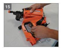
Carefully replace handle assembly. During reassembly, ensure wiring does not get pinched.
