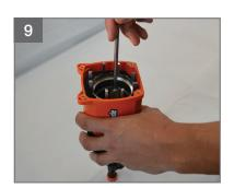
Push drive blade piston assembly to the bottom of the cylinder #24
