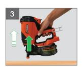
Allow recoil, work contact is released
