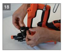
Replace spring #54, bumper #56, magnet #55, housing cover #57 and screws #58
