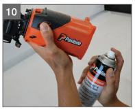
Remove and clean cylinder remove deposits. Always angle backwards to drain correct, avoid washing deposits into lower cylinder
