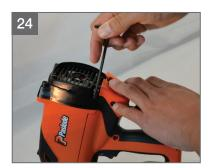
Replace cap #3 and screws #4, tighten
