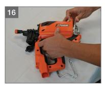
Carefully align head and fan blade. Caution: avoid bending fan blades during reassembly
