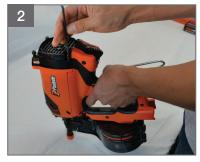
Take off head cap, undo cap screws #3
