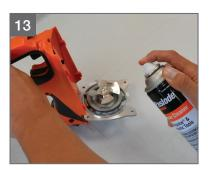
Spray and allow to stand for 30 seconds, then spray off the deposits, use cloth as needed
