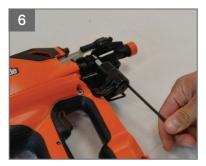
Remove feeder cap screws #58, housing cover, bumping and spring
