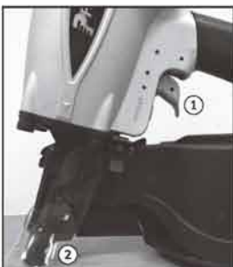
1) Trigger 2) Work Contacting Element 3) Magazine
