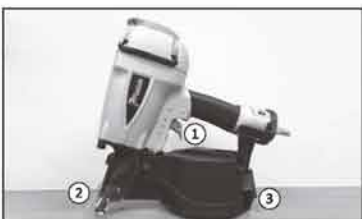
1) Trigger 2) Work Contacting Element 3) Magazine
