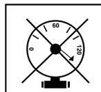
Operate the tool using only the recommended air pressure. Do not exceed the maximum air pressure marked on the tool. Be sure the air pressure gauge is operating properly and check it at least twice a day.
